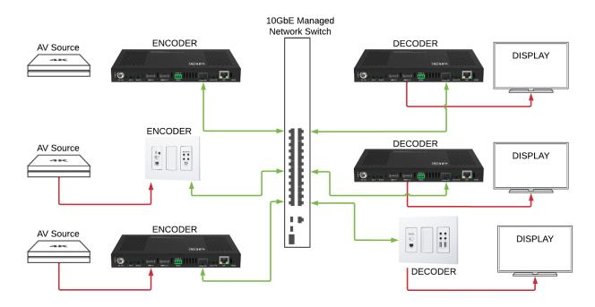
*Note:* Transceiver mode (encoder, decoder or both) can be configured by Arranger server
